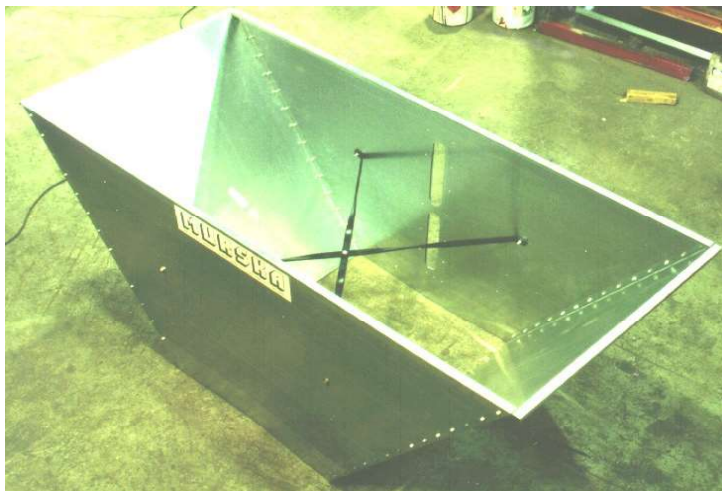
Parts and assembly of extra hopper
