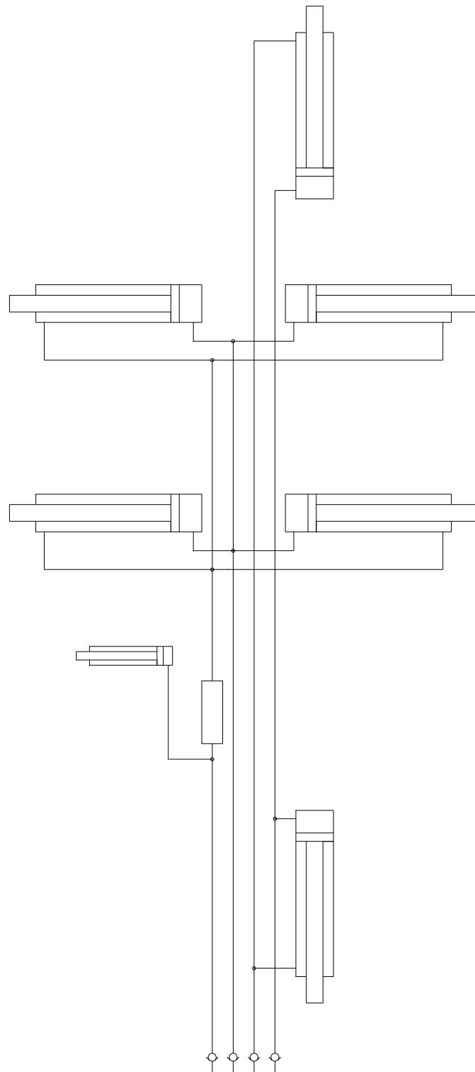
**Syvyyden säädön hydraulikka**
