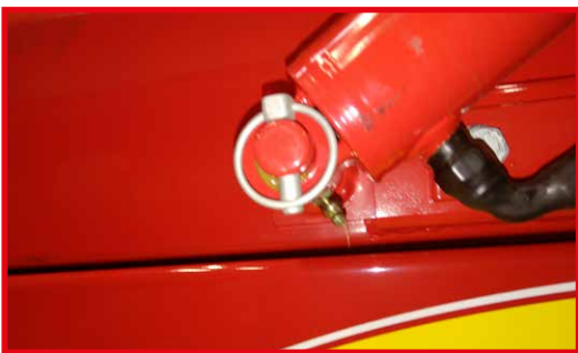
Hinges and ends of cylinder for hydraulic hopper extension.
