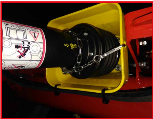
PTO shaft under the spreader: disassemble the PTO shaft and lubricate the 6-grooved ends with grease.
