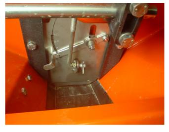
Set the micro-dosing doors at scale 10 on both sides. **Important!** Remember to reset the doors to their original position when spreading fertilizer again.
