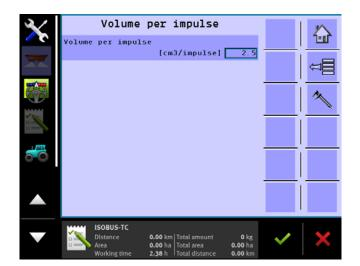
Press Menu / Machine / Calibrations / Volume per impulse. Enter 2.5 and press "Enter".
