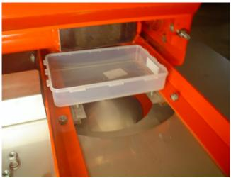
Disassemble the downshutes and place a collection tray underneath each floor belt.
