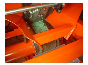
Press the computer's start button and allow the belts to run for a few seconds until material starts flowing down into the collection trays. Stop the spreading.
